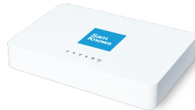
Figure 3: Example of measurement probe: SamKnows Whitebox 8.0 1
